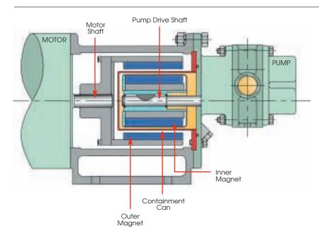
Mag-drive pumps transfer power from the motor shaft to the pump drive shaft via a magnetic coupling. The magnetic coupling consists of an outer magnet and inner magnet, matched in strength. The outer magnet attached to the motor shaft causes the inner magnet attached to the pump drive shaft to turn synchronously with the motor. Since the drive shaft is completely inside the pump housing, there is no need for a dynamic seal and the pumped liquid is completely contained.
