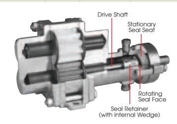
Cutaway view of Sealed Gear Pump showing components of Single Internal Mechanical Seal
