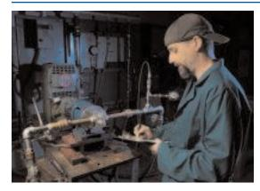
All functional products – including pumps, replacement cartridges and relief valves – are performancetested before shipping. Testing is performed in accordance with Hydraulic Institute standards.
